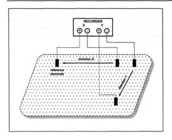
Fig. 2. Measurement of electric field distribution in the ground.
