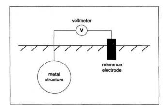
Fig. 1. Potential measurement of structures.
