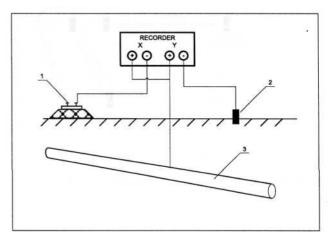
Fig. 4. Method of connection of a recorder to the rail (1), reference electrode (2) and pipeline (3) for measurements by the correlation method.
